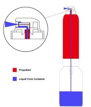
When the button is pressed, propellant and liquid are mixed and dispensed as a spray at the nozzle by action of the venturi effect. Liquid from the jar is pulled up the tube as propellant travels across the holes in the red insert (inside the button). The propellant and liquid do not mix prior to being dispensed out of the nozzle.
